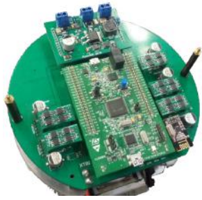
Fig. 5: Picture showing all boards: the kicker module at the top, the stamp module at the center, five motor modules at the sides and one communication module at the corner. Beneath all, the main board.
