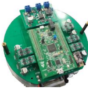
Fig. 2. Picture showing all boards: the kicker module at the top, the stamp module at the center, five motor modules at the sides and one communication module at the corner. Beneath all, the main board.
