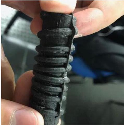
Fig. 8: Roller made with silicon rubber
