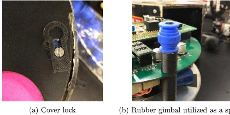
Fig. 10: New mechanism for removal of the cover
