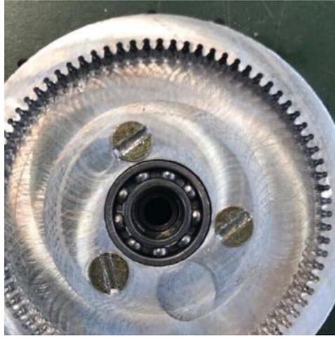
Fig. 6: The machined metal gear.
