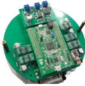
Fig. 8: Picture showing all boards: the kicker module at the top, the stamp module at the center, five motor modules at the sides and one communication module at the corner. Beneath all, the main board.
