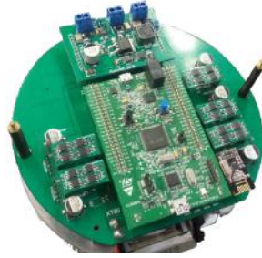
Fig. 12: Picture showing all boards: the kicker module at the top, the stamp module at the center, five motor modules at the sides and one communication module at the corner. Beneath all, the main board.
