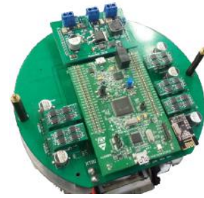
Fig. 2. Picture showing all boards: the kicker module at the top, the stamp module at the center, five motor modules at the sides and one communication module at the corner. Beneath all, the main board.
